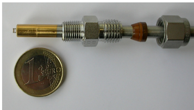
Fig. 1. Fibre probe by ifs-Aachen with diamond prism as internal reflection element.
